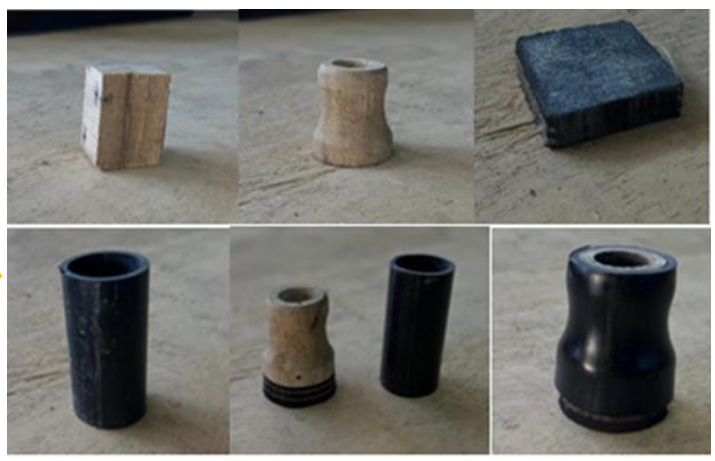
Local end cap manufacturing process (wood, carpet, PVC)
